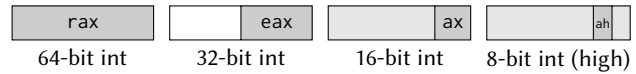
(a) Examples for single element facets (dark gray) of general-purpose registers. For a write-back of 32-bit facets, the upper half of the register is zeroed (white), while for 8-bit or 16-bit facets the untouched part (light gray) has to be preserved via bit masking.
