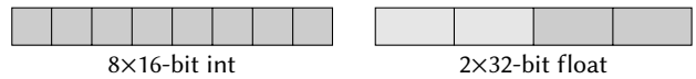
(c) Examples for vector facets of SSE vector registers. Element type and count depend on the instruction, just as the handling of unused parts on write-back.
